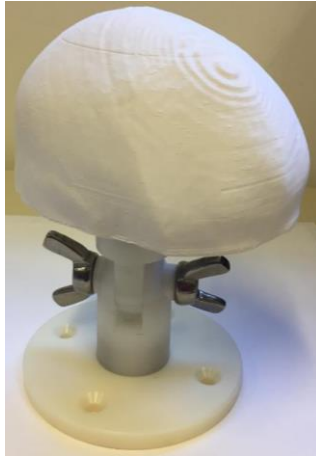
Figure 60. 3D printed skull assembled in the fixation system.
