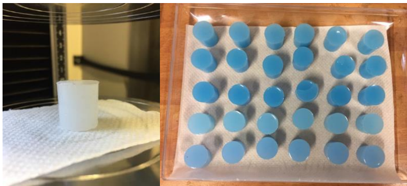
Figure 63. Sample of Contor silicone (left) and samples of Ecoflex® 00-10 (right) before the compression tests.
