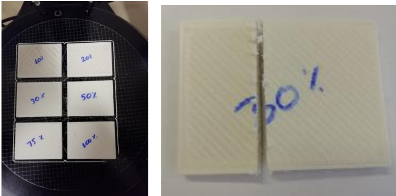
Figure 62. Samples with different infill densities (10, 20, 30, 50, 75 and 100%) to be cut with saw (left) and sample with the selected infill density after the cutting (right).
