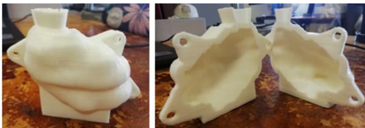
Figure 84. Final 3D printed tumor mold.
