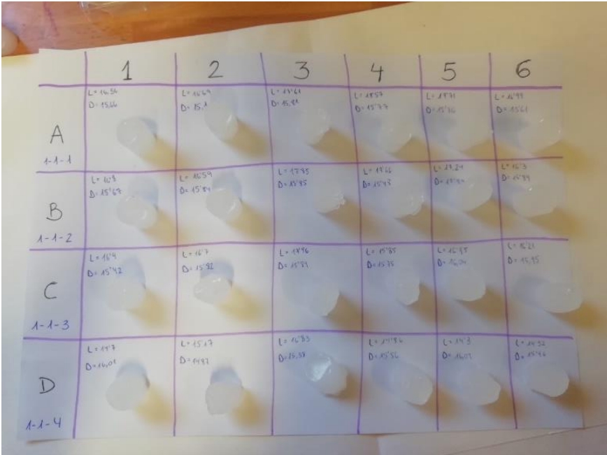
Figure 67. Final silicone samples for the compression tests.
