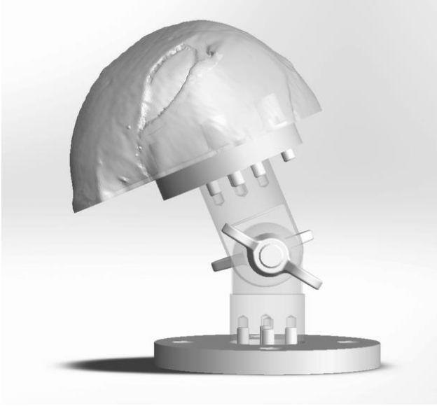
Figure 30. Design of the fixation mechanism of the skull, with adjustable angle and several possible positions of the skull.
