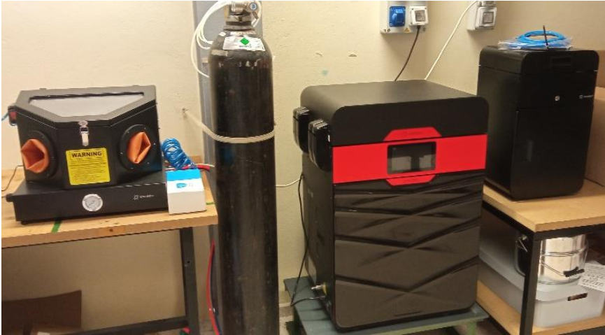
Figure 12. First Selective Laser Sintering machine with desktop format (Sinterit Lisa Pro). Left: sandblaster unit for post-processing. Middle: 3D printer with optional nitrogen atmosphere. Right: sieving unit for material preprocessing (mixing of virgin and reused material and sieving).
