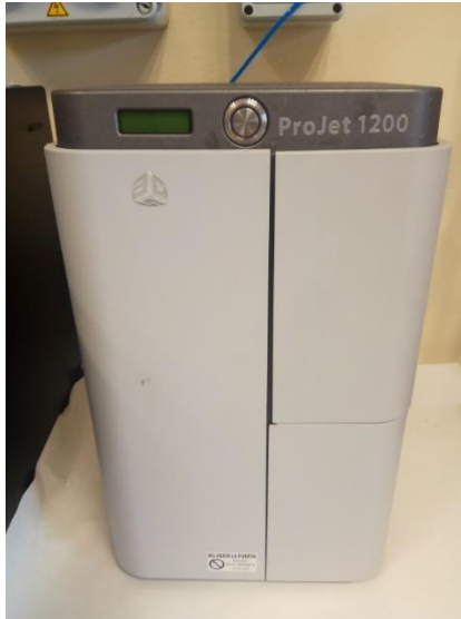
Figure 3. ProJet 1200, vat photopolymerization machine with DLP technology and 'bottom-up printing'.
