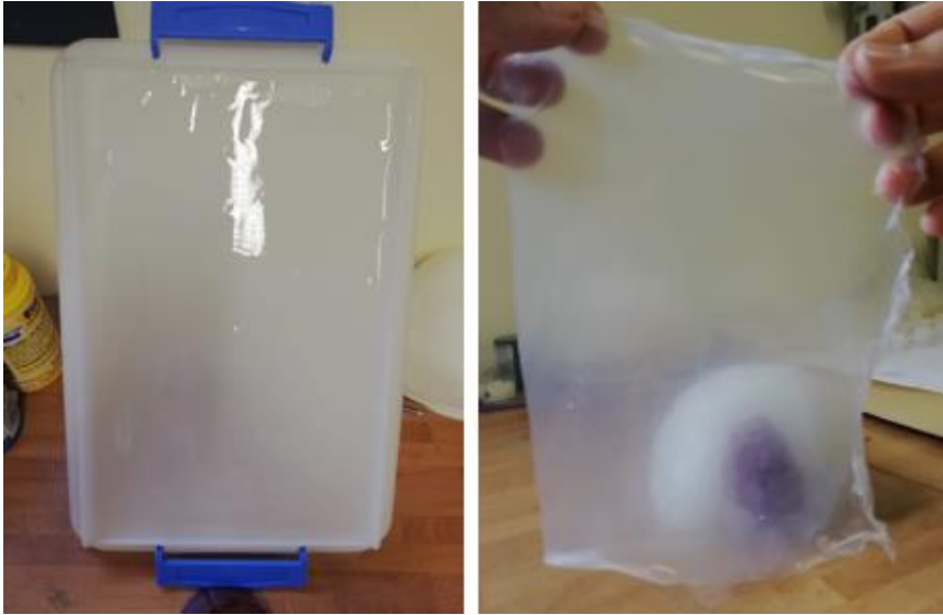
Figure 91. Thin sheet made with 1:1 silicone mixture to simulate the dura mater.
