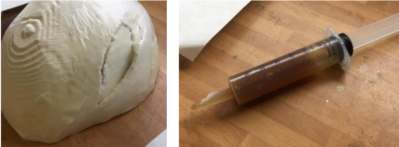
Figure 40. Left: 3D printed model of the final geometry cover with Parafilm® for the leakage test. Right: Syringe with sodium alginate and distilled water (1:20 w/w) to mimic the hematoma.
